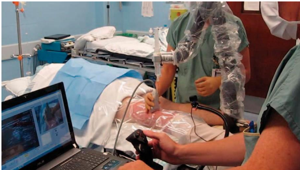
Figure 1.3: The Magellan Robotic System consists of 3 main components: a joystick, a robotic arm and a software control system. Adapted from "First robotic ultrasound-guided nerve blocks in humans using the Magellan system Hemmerling, by Thomas M., et al. 2013, Anesthesia & Analgesia , Volume 116 Number 2, Page 492, with permission from Wolters Kluwer Health, Inc."
